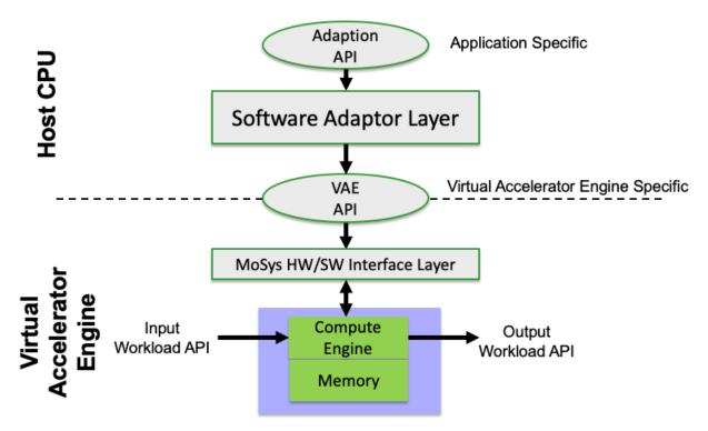
In most cases, there will be a Software Adaption Layer that runs on the host that maps from the application layer API to the VAE API. The adaption layer will perform tasks of mapping or translating from a specific data structure such as machine learning classifier or header look up key into the data structures executed on the available hardware available for the VAE.
