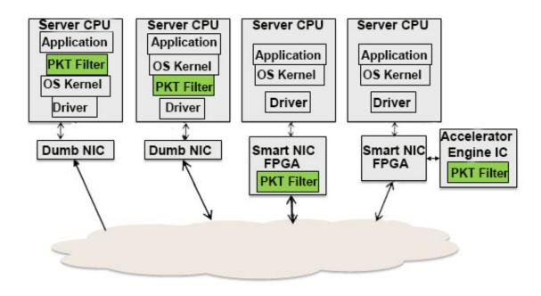
Utilizing the concept of common API and a virtual function, the VAE architecture can be used in hierarchical systems where the exist parallel paths processing packets from a fast path to slower paths. The benefit of the common API is that the same software stack can be used to control each of the paths in the hierarchy in a unified fashion.
