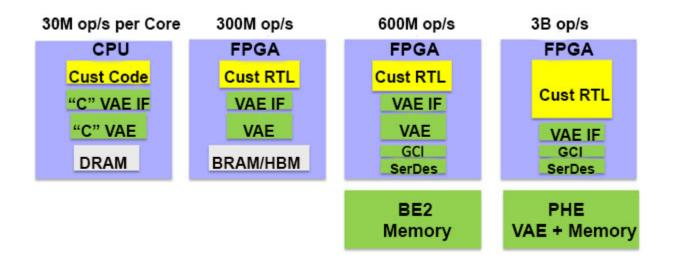
Each VAE platform is designed to support a specific application function such as classify input vectors, indexing databases, or performing optimized calculations where the base function can be generalized enough to fit many types of specific applications.
