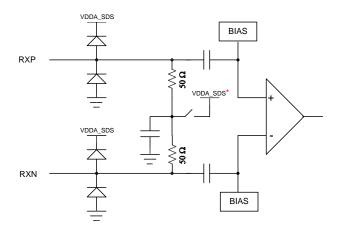
\*Termination common mode can be to VDDS\_SDS (default) or floating.
