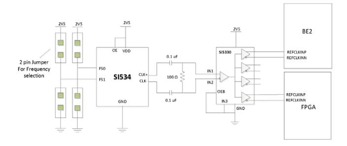
The BE-2 reference clock inputs can be directly driven by any LVDS fanout buffer as long as it meets the jitter and rise time requirements. Please refer to the device datasheet [1] for the actual jitter and rise time specifications. Further, the maximum output common mode voltage of LVDS fanout buffer must be less than 1.3V. AC coupling capacitors should be used at the BE-2 reference inputs if the output common mode voltage of the LVDS fanout buffer is higher than 1.3V.
