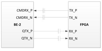
AC coupled using 0.1uF (size 0201) capacitors
